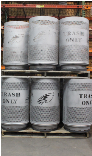
Sandblasted units ready for repair and paint
